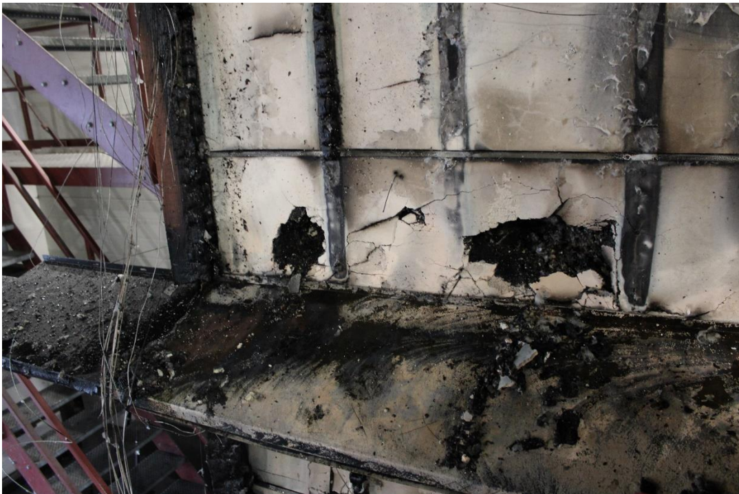
Photo No. 26 Test specimen after the test. Corner below the second flame deflector.
