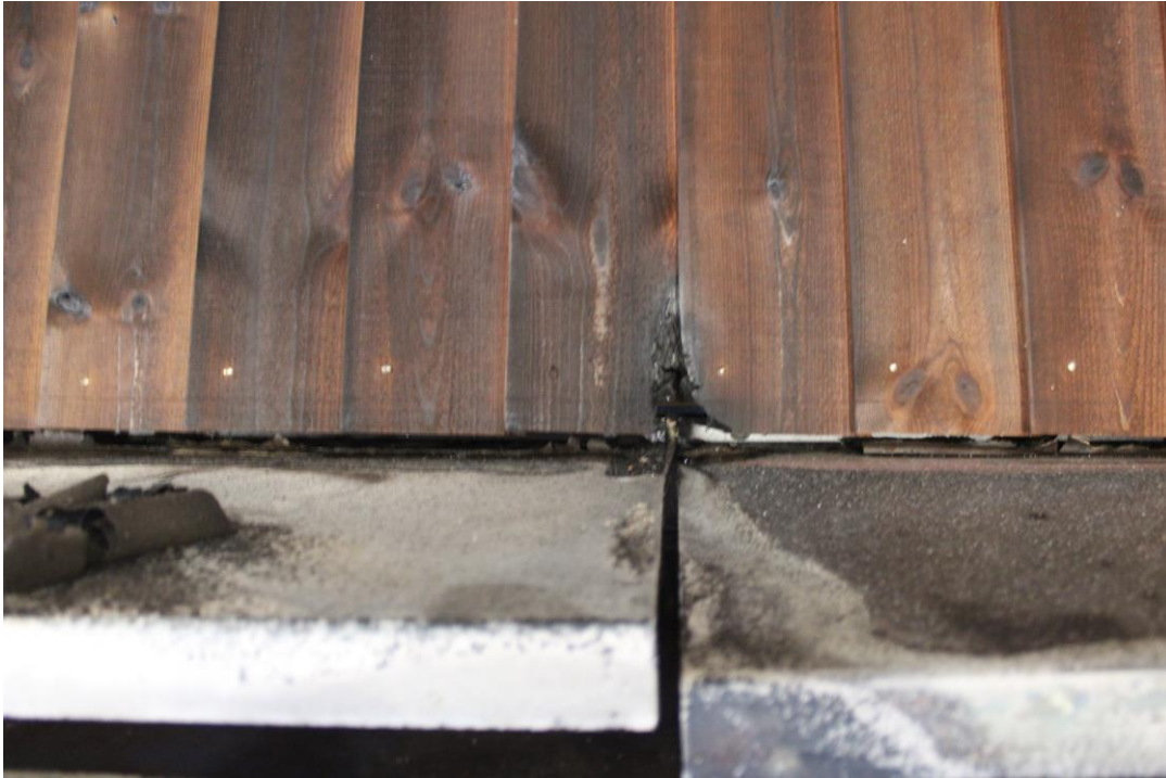
Photo No. 25 Test specimen after the test. Detailed photo above second flame deflector.
