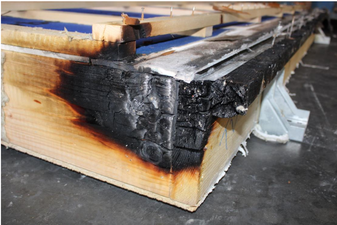
Photo No. 26 Test specimen after the test. Detailed photo of wooden frame corner.
