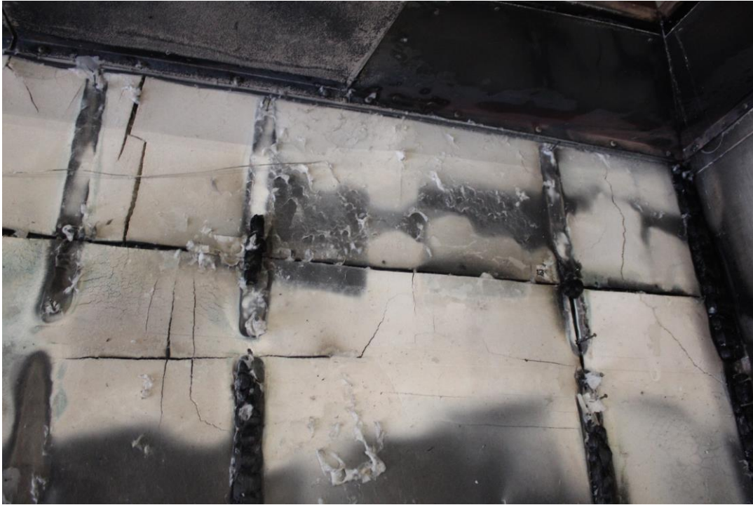
Photo No. 25 Test specimen after the test. Corner below the second flame deflector.
