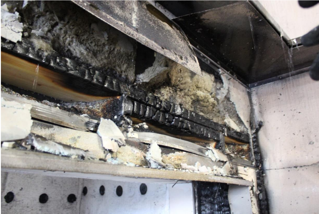
Photo No. 25 Test specimen after the test. Corner below the first flame deflector.
